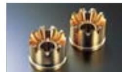
Mold for cold forging (bevel gear mold)
