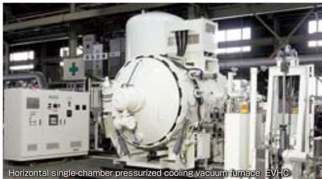
Horizontal single-chamber pressurized cooling vacuum furnace EVHC
