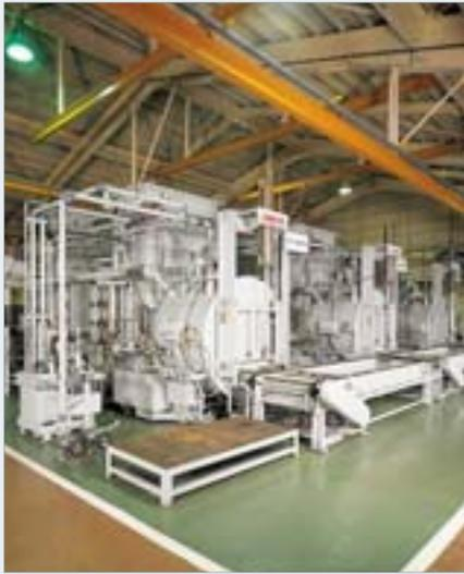
Vacuum purge type triple chamber tempering furnace EVHFD
