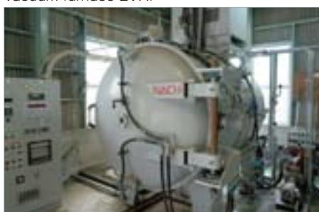
Vacuum purge type triple chamber tempering furnace EVHFD
