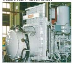
Horizontal single chamber vacuum furnace EVHF
